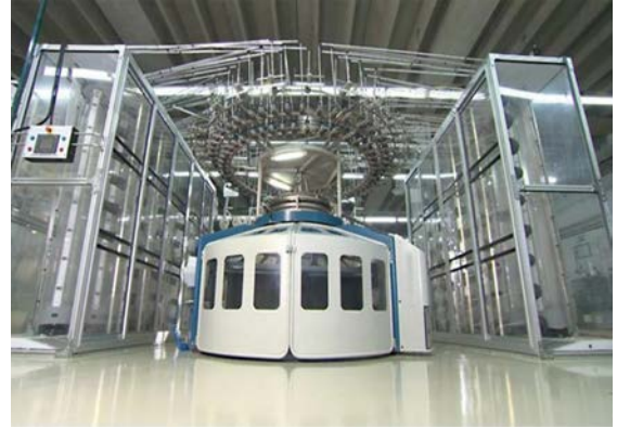
Figure 3: General view of the creel conditioning cabinet that was developed (TPE 2015/03319)
